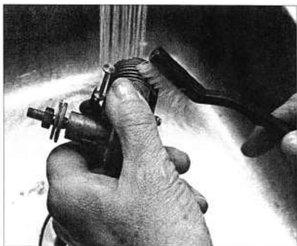
STEP 5 – Using a bristle brush scrub away the baked on oil and dirt. Place a finger over the exhaust and venturi to keep the water out
